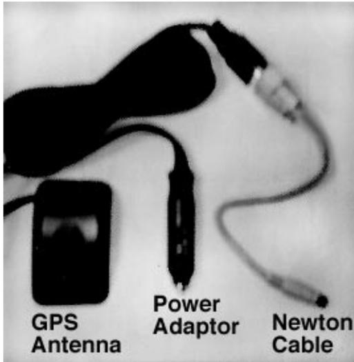
TeleType GPS for Newton includes GPS Antenna, Power Adaptor, and Newton Cable (also includes GPS mounting hardware - not shown)
